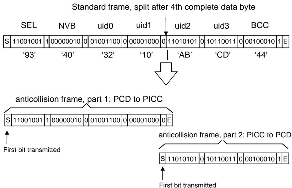
Figure 4 — Bit organization and transmission of bit oriented anticollision frame, case FULL BYTE
