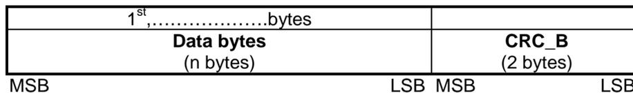
Figure 18 — Position of a CRC\_B within a frame
