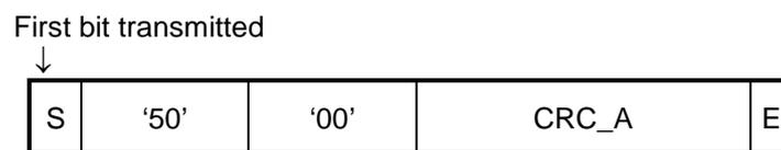
**Figure 7 — Standard frame containing HLTA Command**
