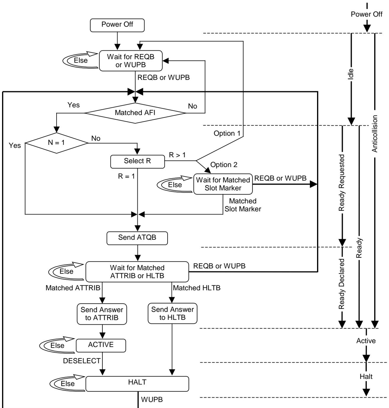
Figure 19 — PICC state transition flowchart example
