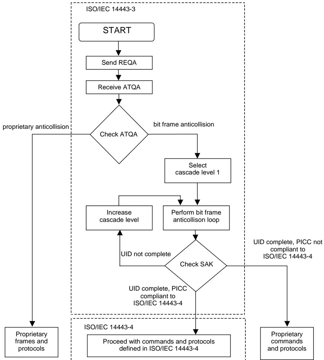
Figure 8 — Initialization and anticollision flowchart for PCD
