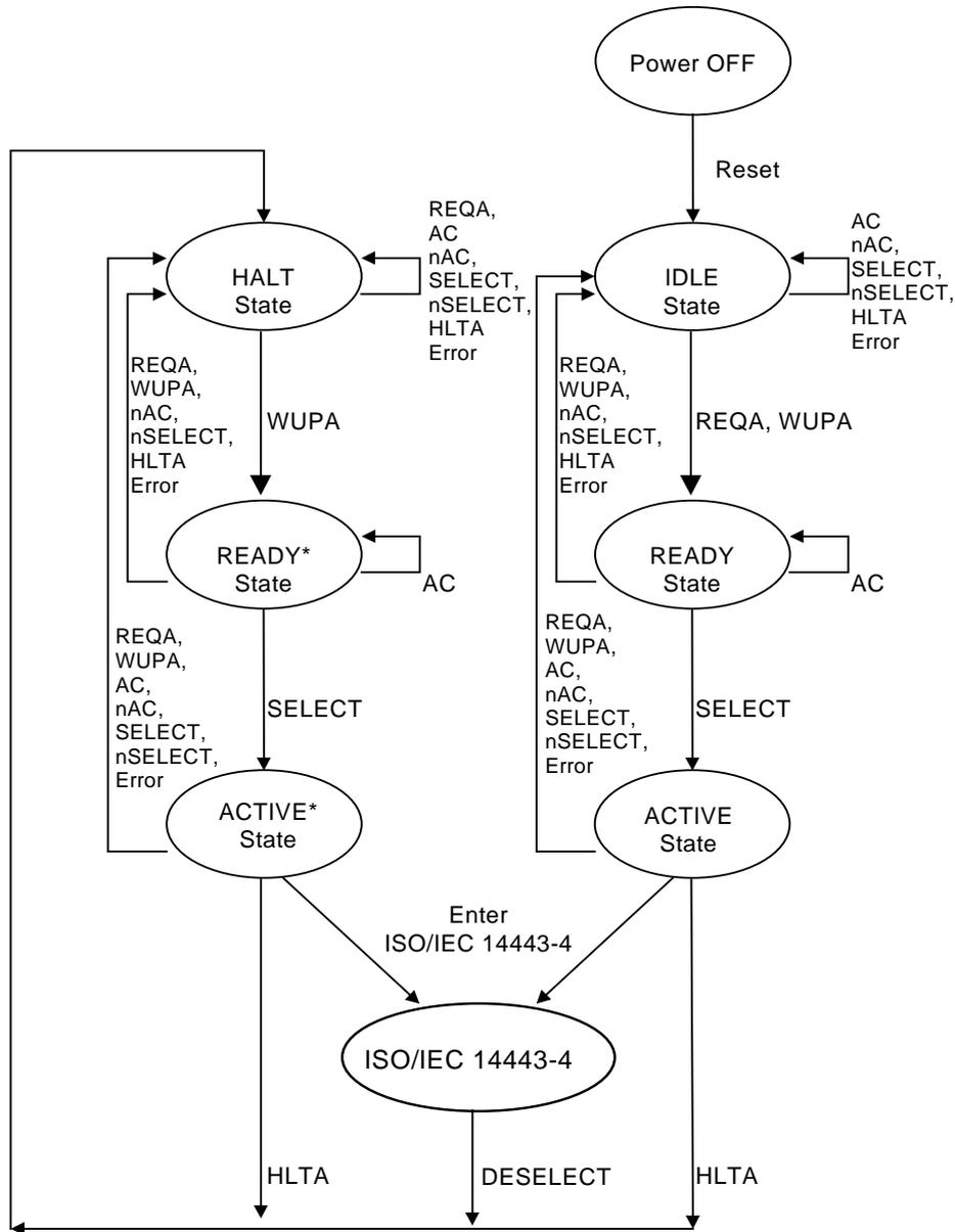
Figure 6 — PICC Type A state diagram
