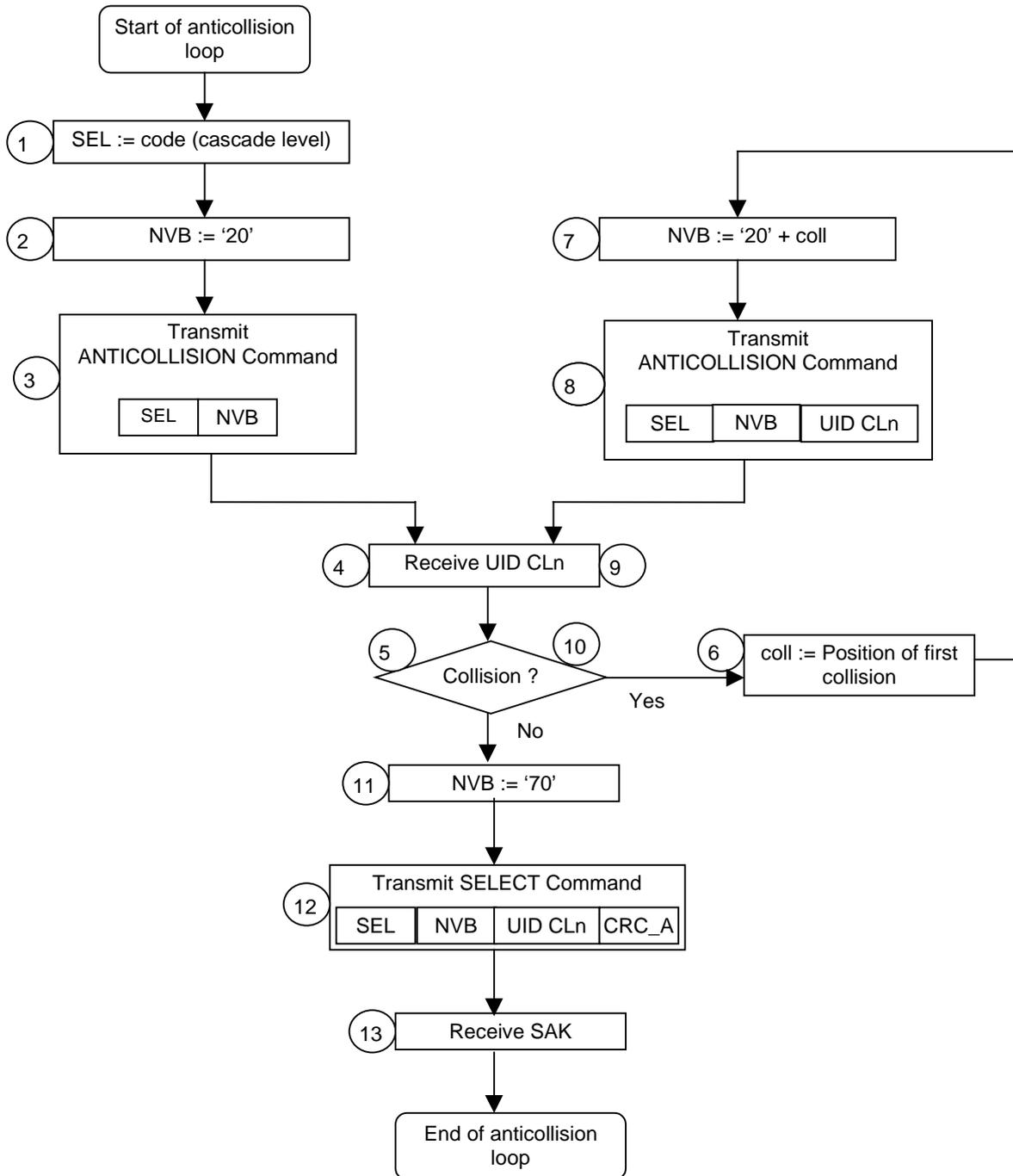
**Figure 9 — Anticollision loop, flowchart for PCD**
