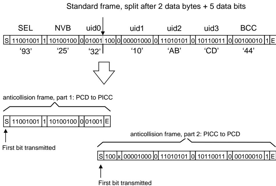
**Figure 5 — Bit organization and transmission of bit oriented anticollision frame, case SPLIT BYTE**
