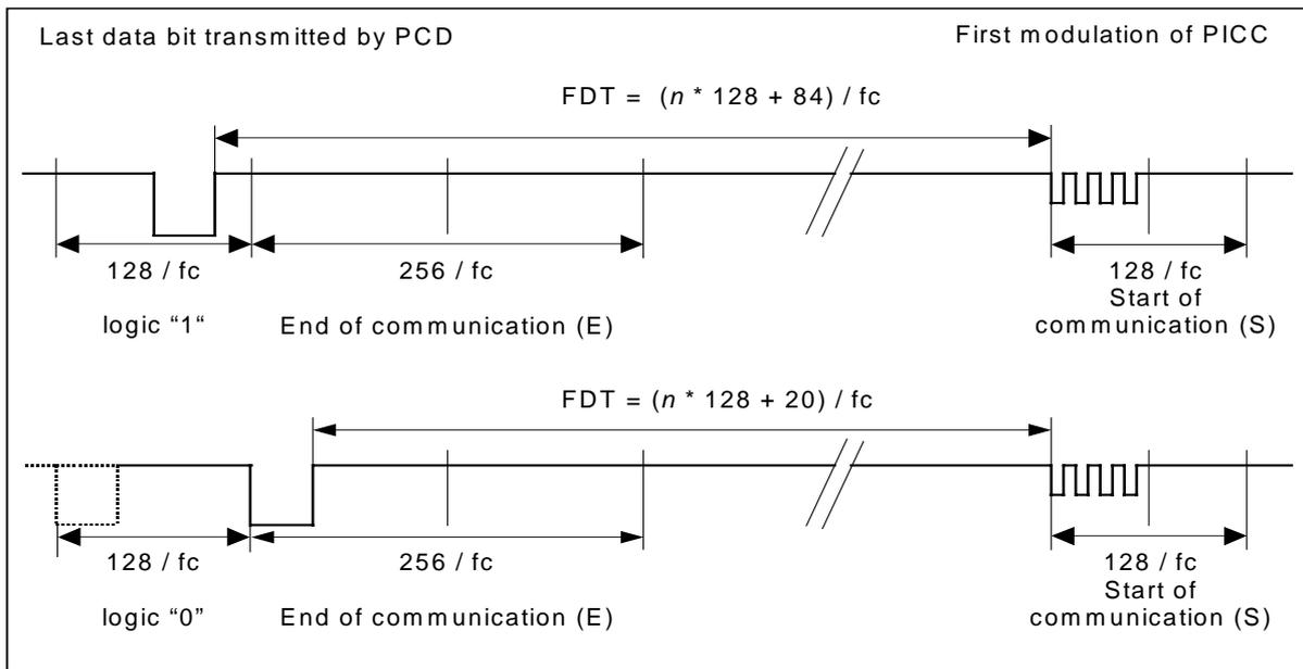
Figure 1 — Frame delay time PCD to PICC
